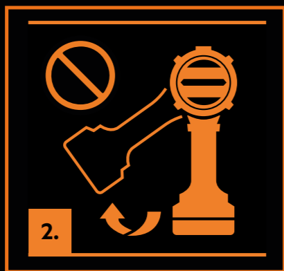
2. ANTI-KICKBACK technology engages & prevents the tool from over-turning
